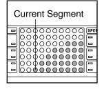
The speed settings for the next seven segments are shown in the seven columns to the right.
